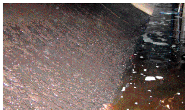
Above left: fuel before and after treatment with an Algae-X fuel polishing system; Above right: fuel production has changed since 1972; Below left: fuel molecules, although tiny, cluster together to form larger particles; Below right: sludge accumulated in a fuel tank
