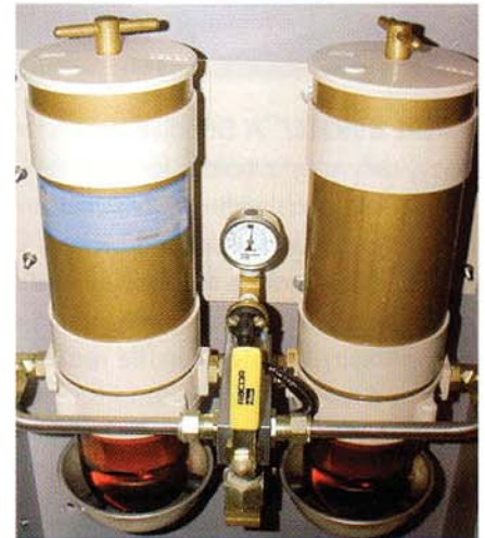
Dual head (duplex) filter arrays allow one filter to be serviced while continuing to operate through the other. Note the sender/switch teed into the vacuum gauge. It's wired to an indicator on the bridge.
