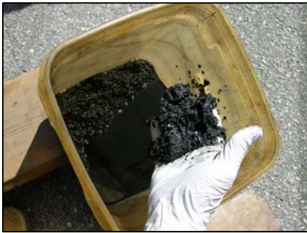
Debris and water removed from the bottom of the fuel/water separator.
